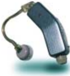
Dahlberg model Magic Ear II, 1957. BTE with miniature external receiver.
